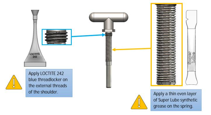
4. Before installing the new T-Handle replacement assembly, ensure both internal threads on housing and external threads on shoulder are clean and free of debris. Insert the new T-Handle into the housing and turn the shoulder clockwise until the shoulder is fully seated on the housing. Since the threads will be secured by the LOCTITE, use the recommended tool to slightly tighten the shoulder (Do not over tighten).
